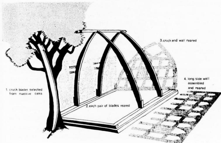
PLATE I. Newton Hall: the sequence of a cruck frame construction.
