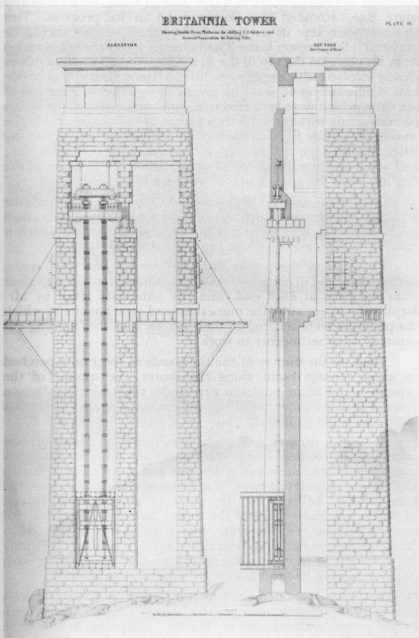
Britannia Tower. Shewing Double Press, Platforms for shifting A 2 Girders, and General Preparations for Raising Tube (From Britannia & Conway Tubular Bridges by Edwin Clark)
